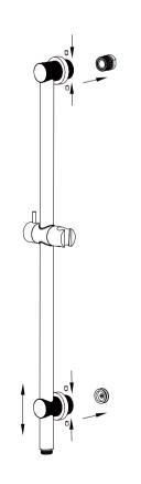
4. Push shower rail assembly onto the wall/tile face.
