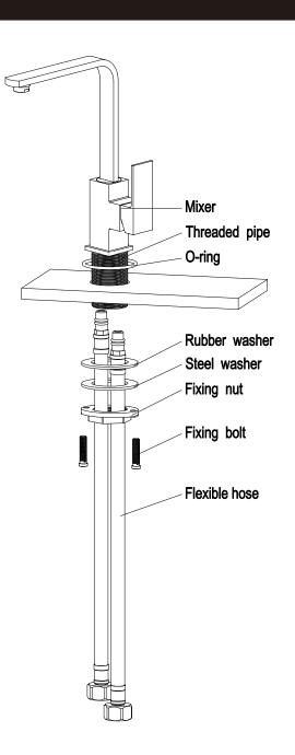
1.Screw the flexible hoses and fixing bolt into the mixer body, and fully hand tighten.
