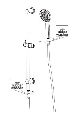
5. Connect shower rail and hand shower with hose. TEST & CHECK FOR LEAKS.
